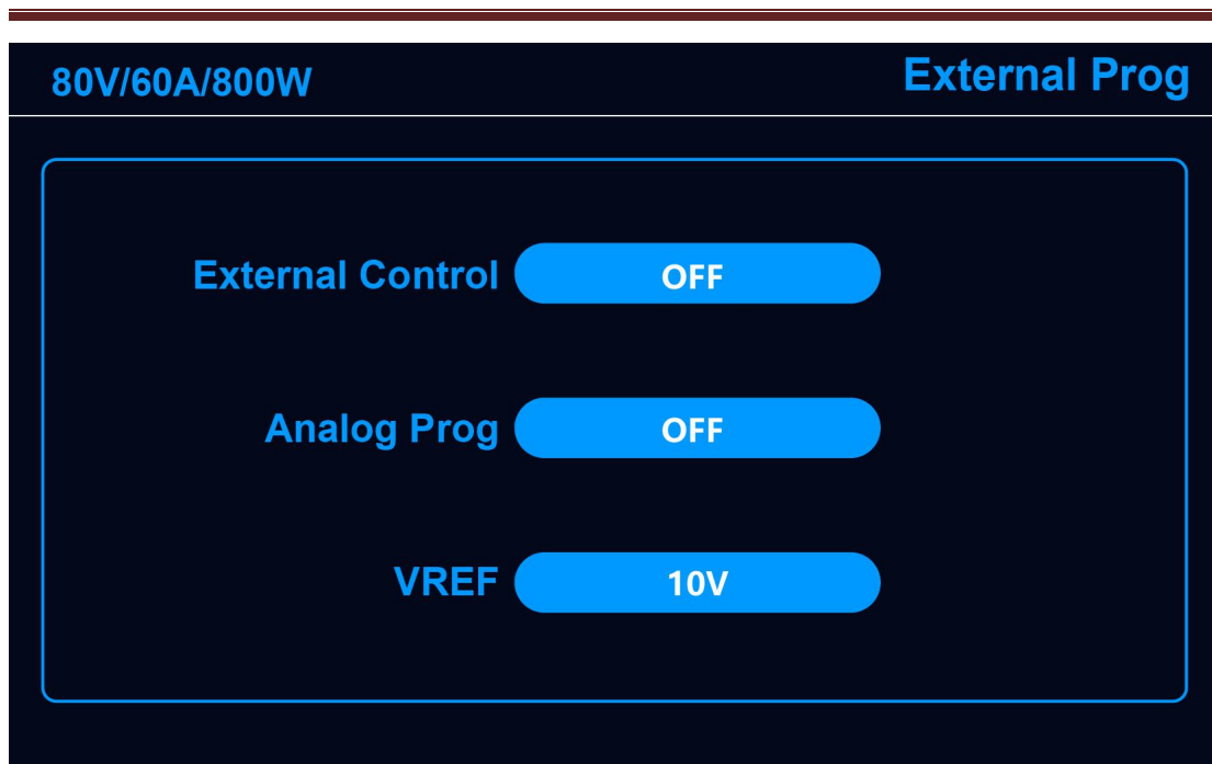
Figure 31 External Prog Interface
