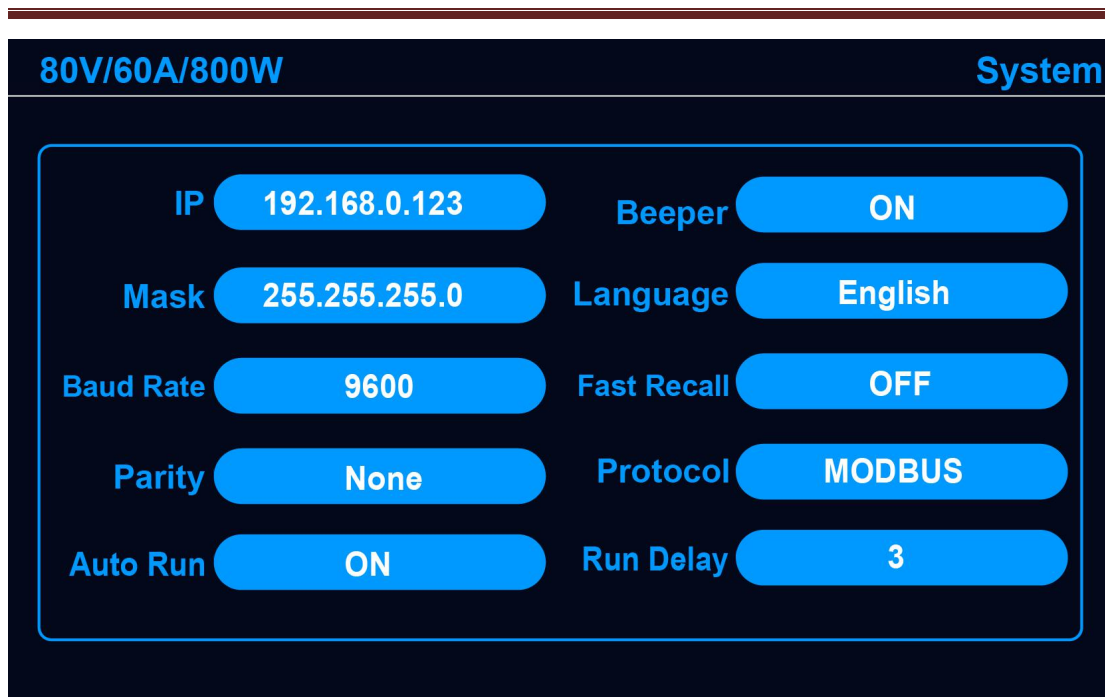
Figure 40 System Configuration Interface
