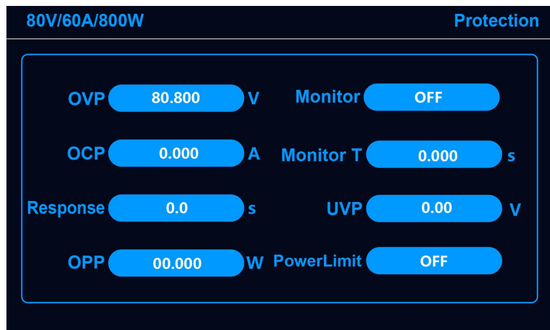
Figure 30 Protection Setting Interface
